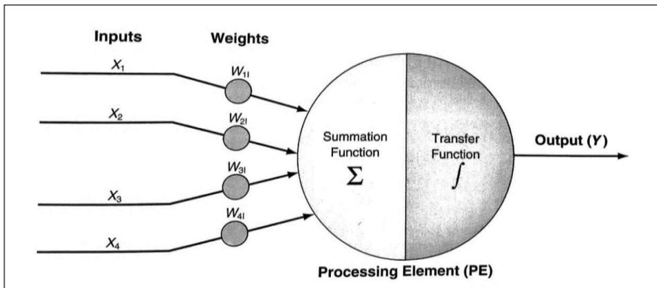
**Figure 6.** Processing Information in an Artificial Neuron
